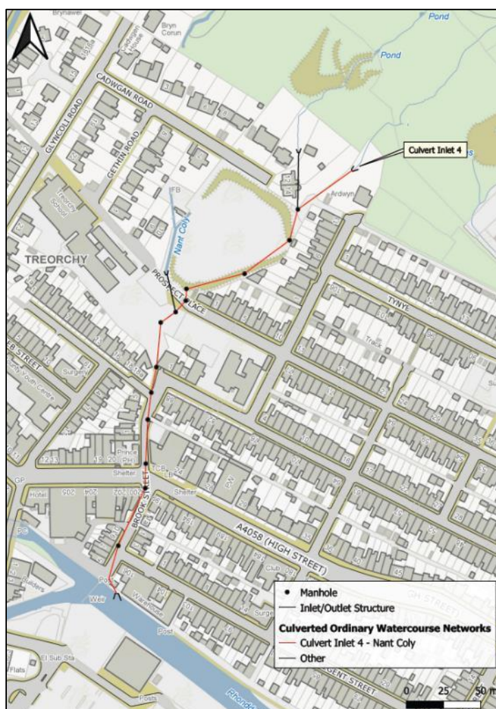
Figure 17: Surveyed culverted ordinary watercourse network within the 'Nant Coly' sub-catchment
